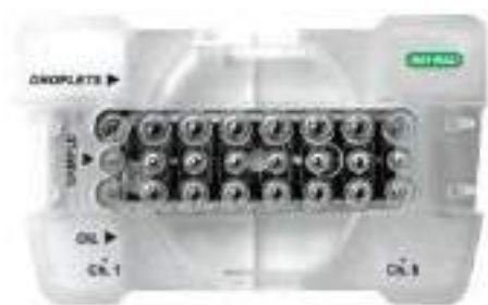
Figure 17 Image of the DG8™ cartridge used to create the emulsion (Droplet Digital™ PCR – Application Guide).
